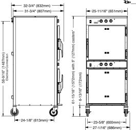
$^*60\text{-}11/16"$  (1540mm) - with optional 3-1/2" (89mm) casters  $^*62\text{-}1/8"$  (1577mm) - with optional 6" (152mm) legs
