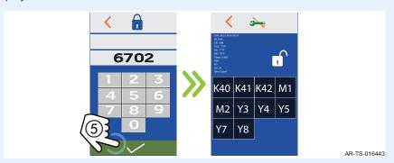
5. **Touch** the designation for the component to be tested. The box will turn green indicating the component is being energized.
