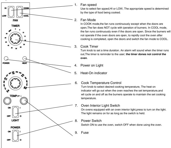
The fan speed can be set to high or low speed by placing the FAN HI/LOW button to the desired setting.
