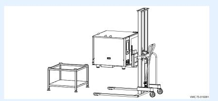
2. **Lower** the oven onto the stand. **Make sure** the legs fit into the pockets on the stand.
