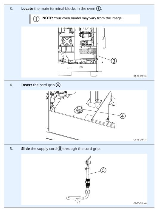
6. **Install** the supply cord into the oven far enough to reach the ground terminal block.
