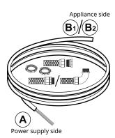
Remove enough cable covering so that wires reach the terminal blocks. Depending on the application, install the straight or the elbow fitting on to the cable.
