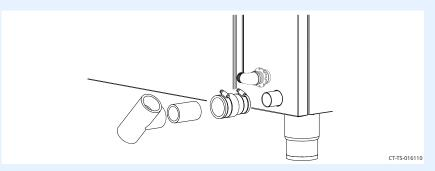
3. **Cut** a short piece (3.25" minimum) of drain pipe and install a 45° elbow into the Tee fitting. Install the vent pipe into the elbow fitting.
