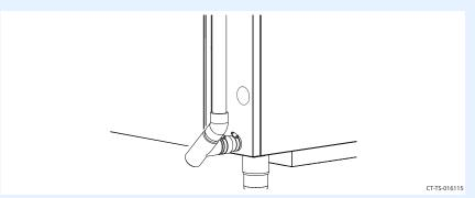
4. **Install** the 45° elbow to the Tee. **Install** the drain pipe. **Install** the 90° elbow. **Secure** the drain pipe with the clamps and straps in the kit.
