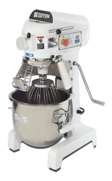
Planetary Mixer, Floor Model, 20 Quart Capacity, 3 Speeds, Gear-Driven Motor, Timer, Emergency Stop, Manual Bowl Lift, Includes Stainless Steel Bowl, Safety Guard with Integrated Feed Chute, Dough Hook, Whip & Flat Beater, #12 Hub, Cast Iron Frame with Enamel Coated Metallic Gray Finish, 1/2 HP, 120V/60/1P/1.44kW/12A, NEMA 5-15P, NSF, cETLus, ETL-Sanitation
