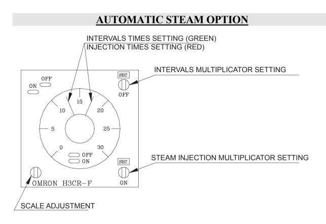
By pushing the GREEN button, the button will light up and the automatic system injection will start. The injection will be done as per the pre-adjustment time on the automatic steam timer. The standard steam timer (white light) will light up during the steam injection. Push the RED button to stop the automatic steam injection and then, the GREEN button will turn off.
