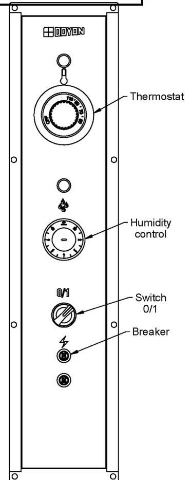
**When the proofer is not in operation, open the doors to let out the humidity and to prevent mould.**
