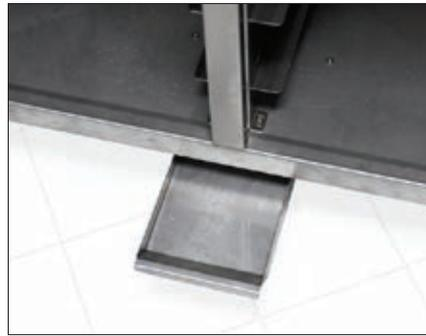
Remove the water from the container on a monthly basis.
