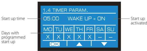
Use the **(B)** or **(C)** buttons to select the start time and the **(A)** button to validate. Use the **(A)** button to select the START-UP PARAMETER and activate the ON position. Use the **(A)** button to select the weekday and the **(B)** or **(C)** button to validate the chosen option, according to the following scheme:
