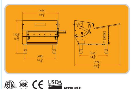
**Rollers:** 3.5" (9cm) dia. by 15" (38cm) length **Scrapers:** Synthetic, Spring Loaded, Removable
