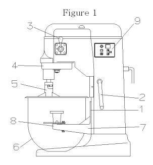
The GEAR SHIFT LEVER (figure 1-3) is used to change speeds. Always stop the mixer before changing speeds. To change speeds, turn the switch OFF, move the gearshift lever to the desired speed, and turn the switch back ON.
