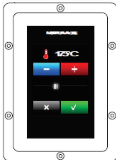
Setting the operating set point.
