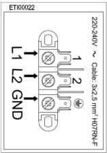
carry out these operations. The appliance must be connected to the mains using a H07RN-F cable or equivalent.
